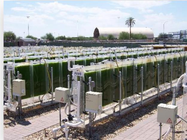
Flat-plate "Acrylic" Photobioreactors. Photo by AzCATI: http://asulightworks.com/blog/azcati-update-plastic-film-vs-acrylic-photobioreactors
