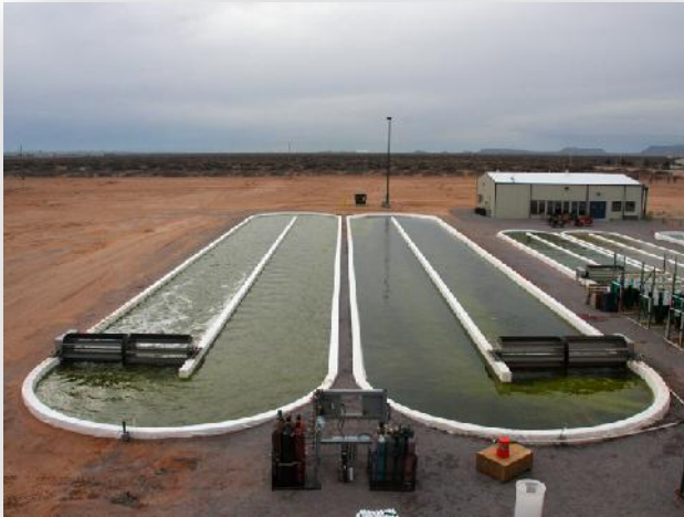
A pair of 200-foot algae open ponds at Sapphire Energy's Las Cruces, New Mexico R&D Facility. Photo courtesy Sapphire Energy.
